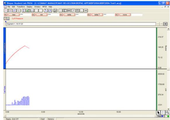
*TIP A generally accepted application is that for each animal, 10 measurements are recorded and mean values are calculated. In the append mode, 10 consecutive measurements can be made in the same file.*
