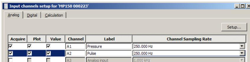
3. Enable analog inputs A1 and A2 and select the Acquire, Plot and Value options.
