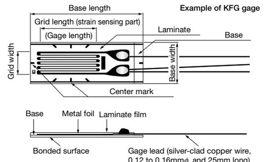
The strain gage is bonded to the measuring object with a dedicated adhesive. Strain occurring on the measuring site is transferred to the strain sensing element via the gage base. For accurate measurement, the strain gage and adhesive should match the measuring material and operating conditions including temperature. For the method of bonding the strain gage to metal, refer to Page 8.
