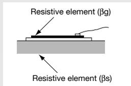
The self-temperature-compensation gage is designed so that  $\epsilon_T$  in the above equation is approximated to zero by controlling the resistive temperature coefficient of the gage's resistive element according to the linear expansion coefficient of the measuring object.
