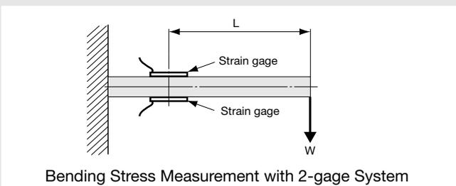
Bending Stress Measurement with 2-gage System
