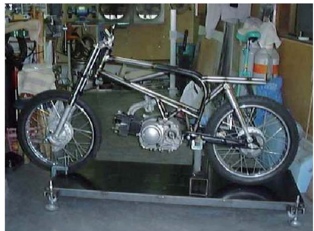
Photograph 3 Finished Pipe Frame Assembly
