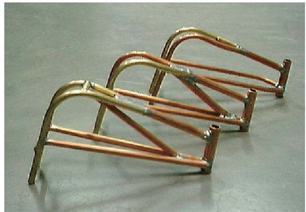
Photograph 2 Pipe Frames Designed with Different Reinforcements
