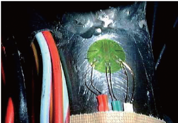
Photograph 4 Condition of Attachment of 3-axis Rosette Gages
