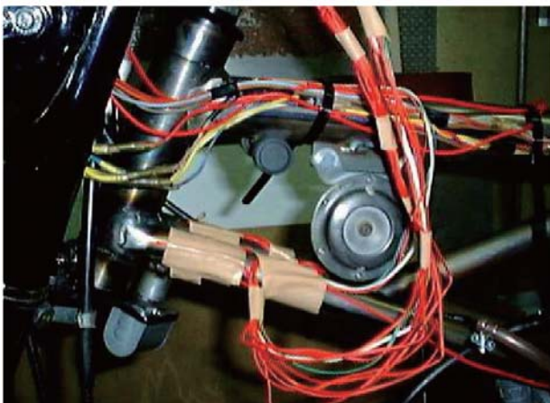
Photograph 5 Condition of Wiring of Gage Leads
