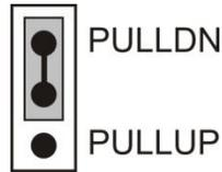
Figure 6. Pull-down jumper
