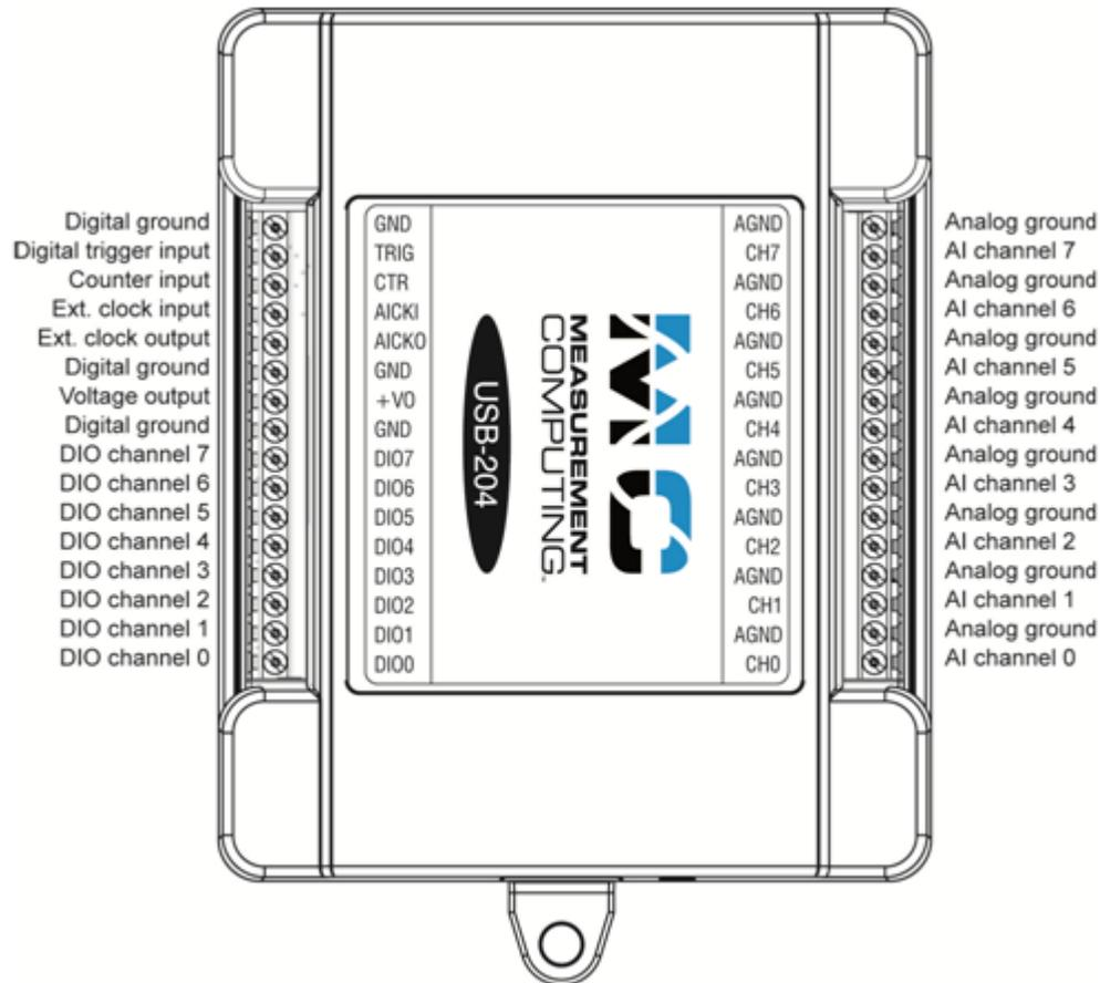
Figure 3. USB-204 pinout
