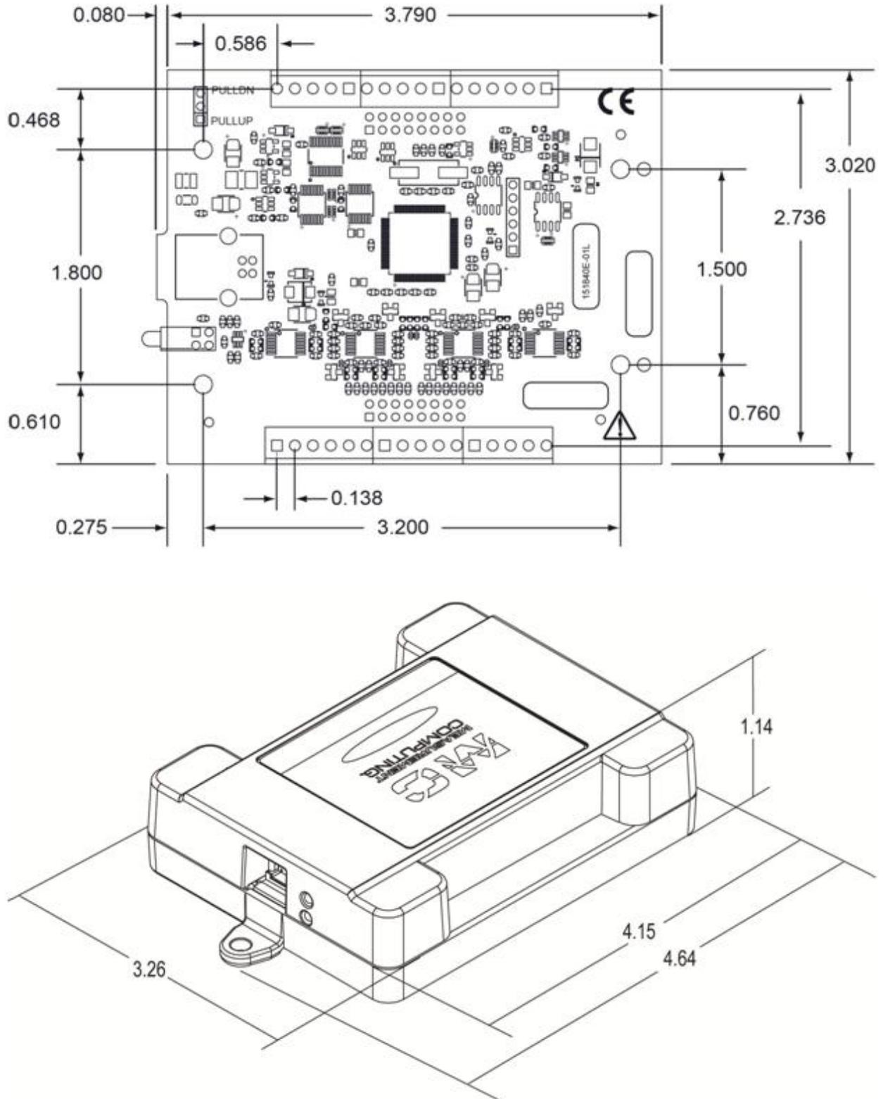
Figure 7. Circuit board (top) and housing dimensions
