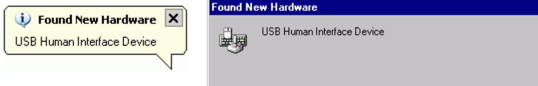
After the USB-3106 is installed, the popup balloon or dialog states "Your new hardware is installed and ready to use," and the power LED should flash and then remain lit. This indicates that communication is established between the USB-3106 and your computer.
